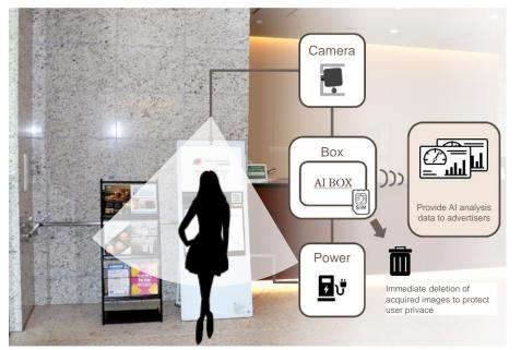
Edge AI cameras on installed on signage to analyze viewing behavior and provide data to advertisers
